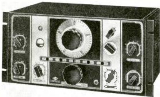
Front view of the new National NC-100 receiver which uses 12 tubes. It has band-switch and indicator, tuning lamp, and a dial which gives extraordinary band-spread.
