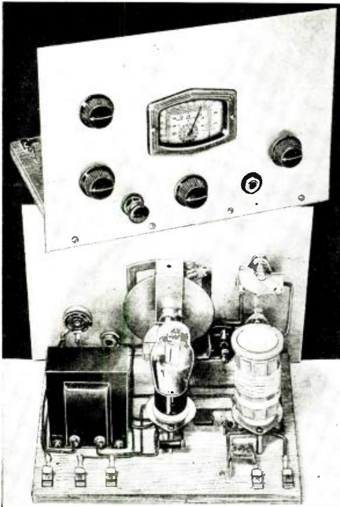
European stations can be heard easily with a pair of headphones on this "one lugger." A single 19-tube gives 2-tube performance—acting as the detector and also as one stage of A.F. amplification.
